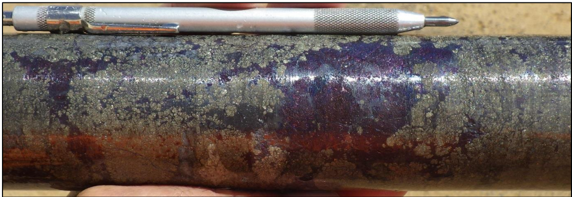
Photo 3. Chalcocite(+digenite)-bornite-covellite veining at 859.0m in SMD044W1 (This photo is of the other side of the core in the previous photo).
