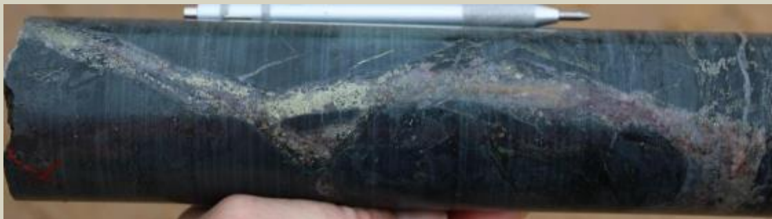
Anhydrite-magnetite-chalcopyrite veining in sediments at 594.9m.
