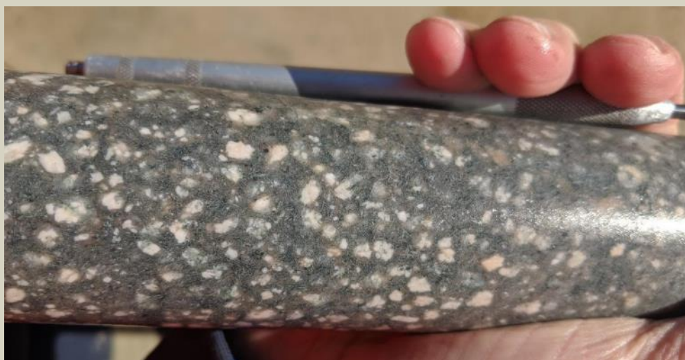
QDP with well developed disseminated actinolite magnetite epidote alteration at 1605.8m.
