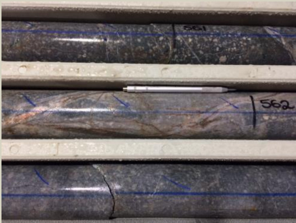
Quartz and anhydrite veining at 562m.
