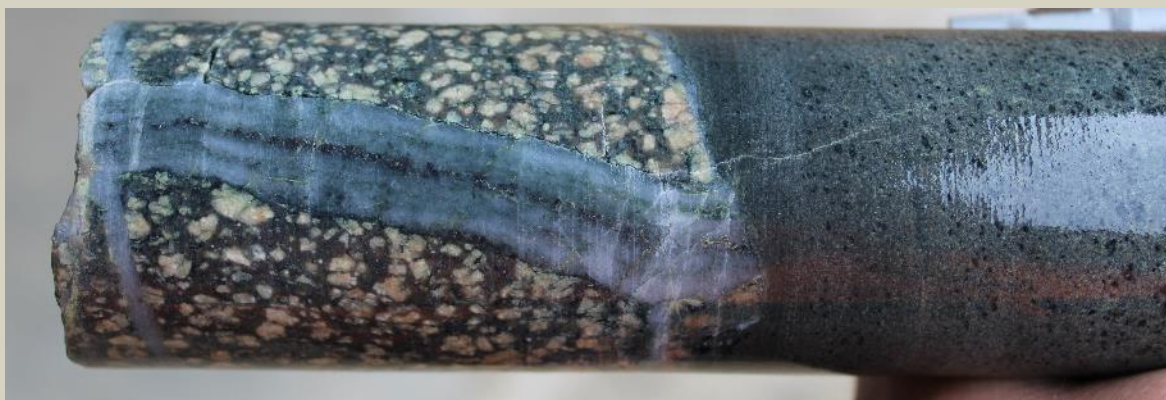
Laminated quartz-magnetite vein (with central magnetite seam) in QDP cut by a micro gabbro dyke at 1510.0m
