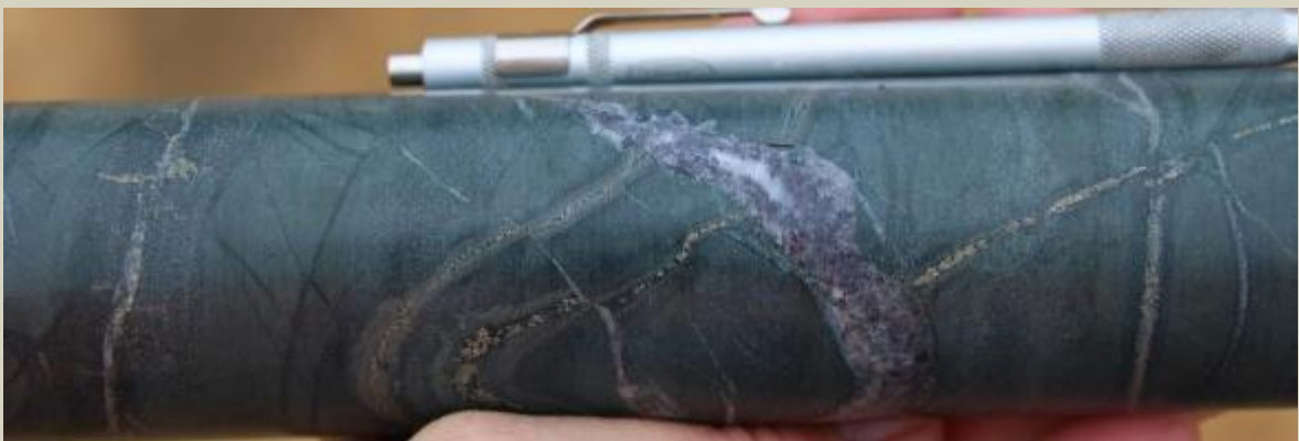
Carbonate-hematite-anhydrite vein cutting pyrite D veins in siltstone at 1190.5m.
