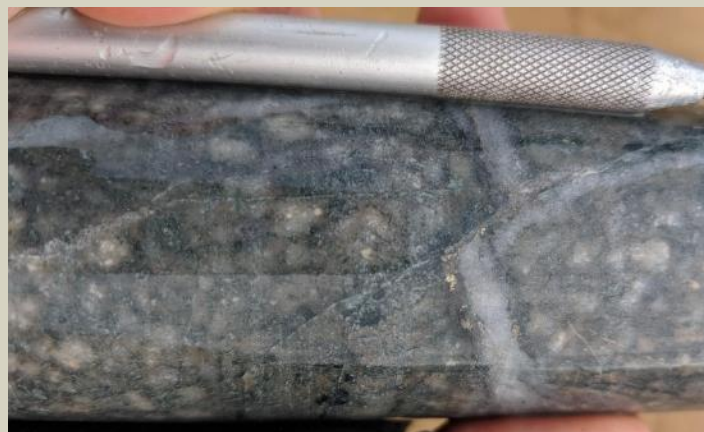
Railroad M vein with trace chalcopyrite in margin at 1581.4m.
