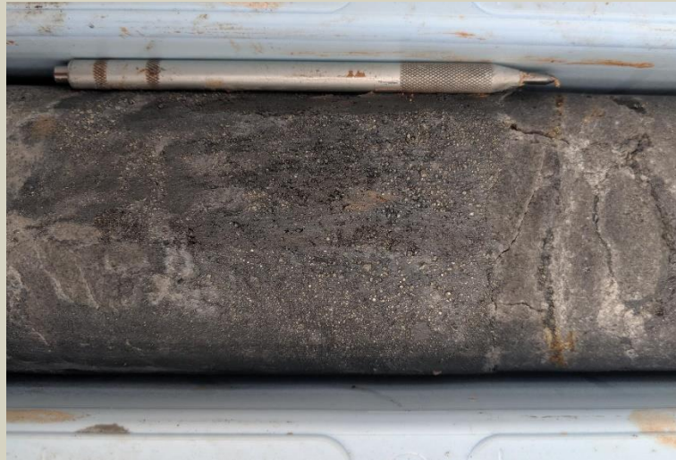
Pyrite + chalcocite in fracture near the base of oxidation at 24.8m.
