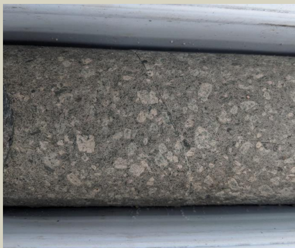
Course grained dacite porphyry at 98m.
