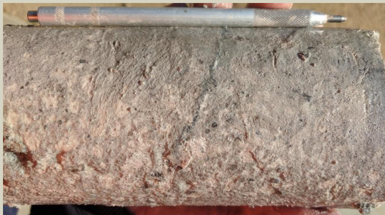
Clay altered coarse grained dacite porphyry at 35m.
