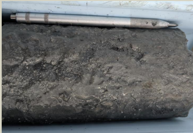
Weathered clay with quartz and pyrite at 84.4m.
