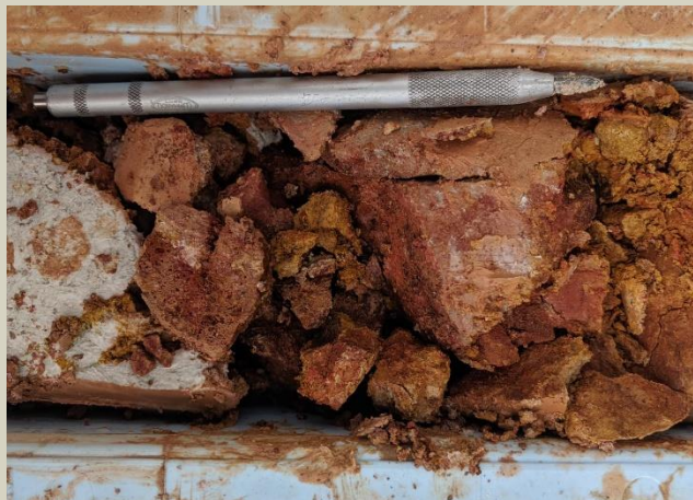
Limonite/hematite stained fractures in leached zone at 22.4m.
