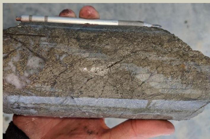
Massive pyrite and quartz veining at 86.5m.
