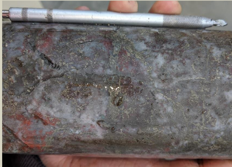
Massive quartz pyrite hematite veining at 92m.
