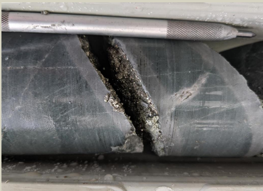
Pyrite D vein in green altered sandstone at 155.6m.
