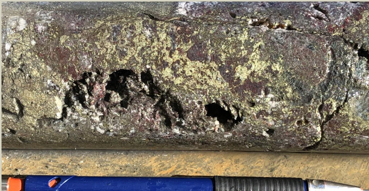
Hematite+chalcopyrite>>pyrite+quartz, vuggy semi-massive sulphide. 201.9m
