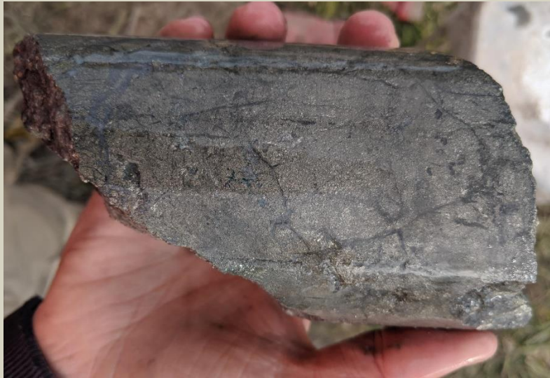
Massive pyrite vein at 83.4m
