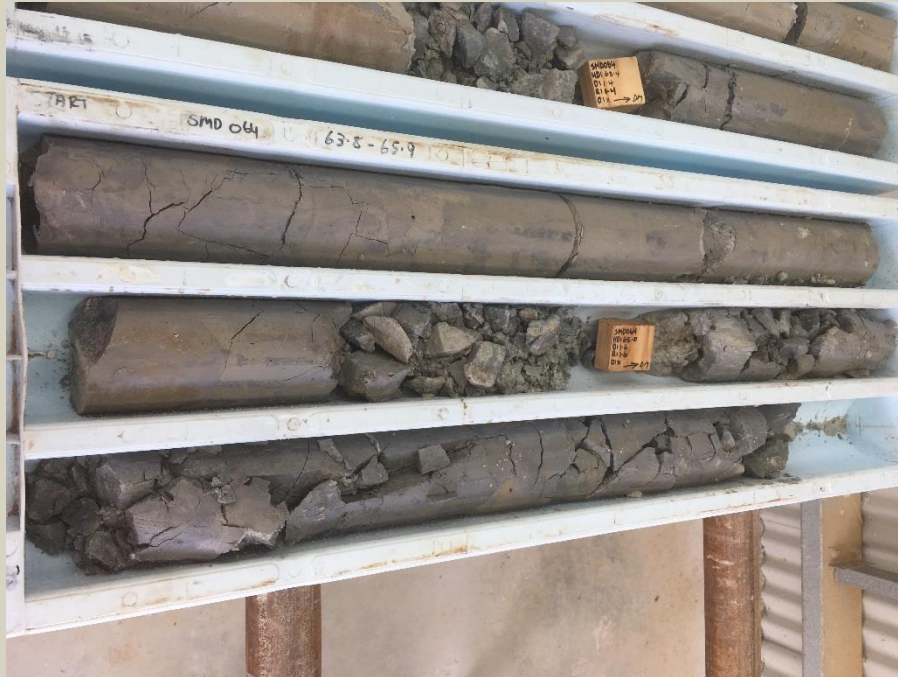
Clay altered sandstone at 63.0m.
