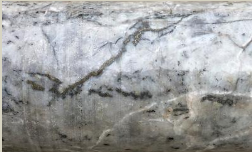
Intense pervasive dolomite+quartz+talc, cut by pyrite stringers. 149.1m
