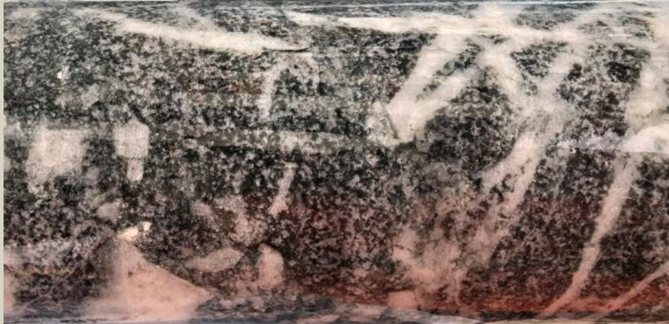
Gabbro / ultramafic intrusive cut by quartz stockwork veins. 93.2m
