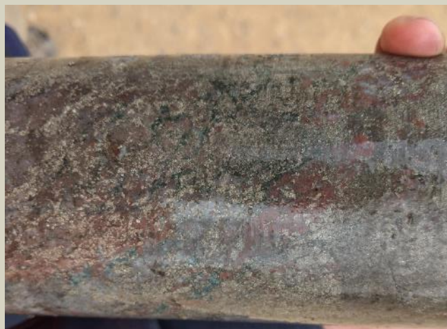
Quartz hematite pyrite vein zone at 82.7m.
