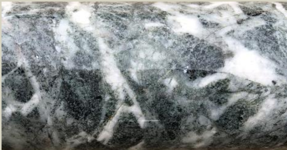
Fragmented quartz+carbonate veins in chlorite+quartz-altered ultramafic. 157.1m
