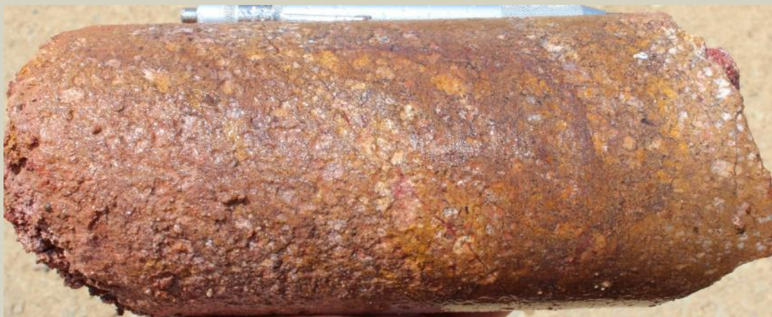
Weathered dacite at 7.8m
