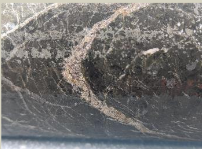
Anhydrite pyrite chalcopryite vein at 118.8m.
