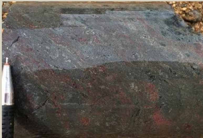
Banded massive sulphide, mostly pyrite with minor chalcopryite and hematite. 29.7m
