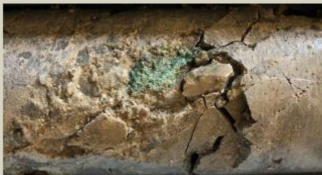
Tuffaceous siltstone, strong pervasive sericite+clay with patch of green clay. 49.3m
