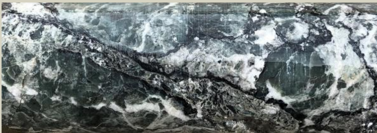
Breccia vein within a brecciated serpentinite with talc+serpentine+dolomite. 173.9m
