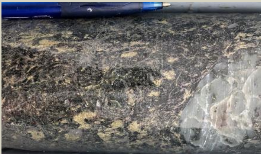
Coarse grained blebby chalcopryite, together with galena and sphalerite in a coarse sandy unit within the serpentinite. 108.1m
