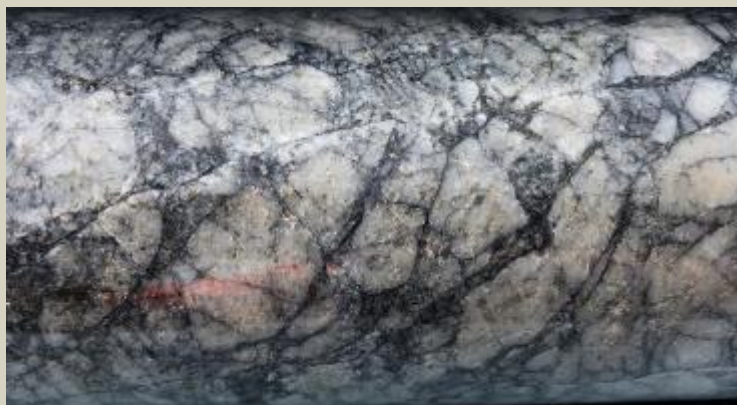
Tonalite-clast breccia with jigsaw-fit texture. 75.0m. Represents a tectonic breccia and/or autobreccia.
