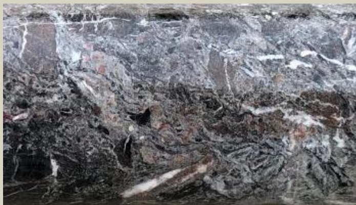
Serpentinite-clast breccia with weak to moderate pervasive carbonate+hematite. 173.1m
