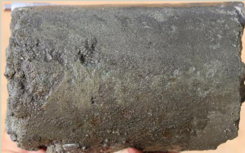
Massive pyrite+chalcopyrite vein at 70m
