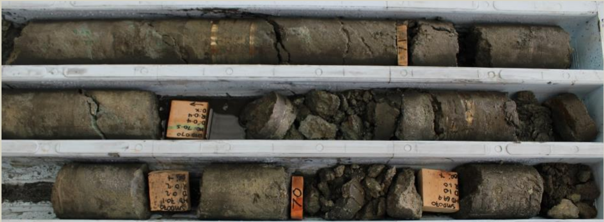
Massive sulphide veining at 70-71m.
