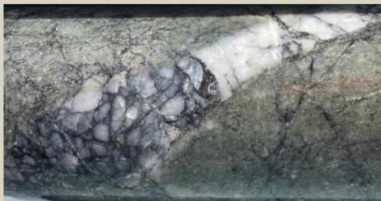
Fractured aplite / quartz vein in tonalite. 69.1m
