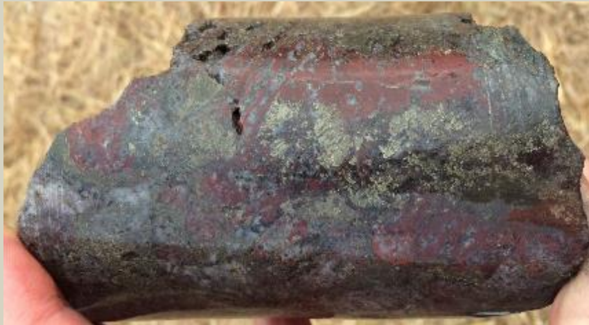
Quartz-pyrite-hematite-chalcopryite vein at 29.0m
