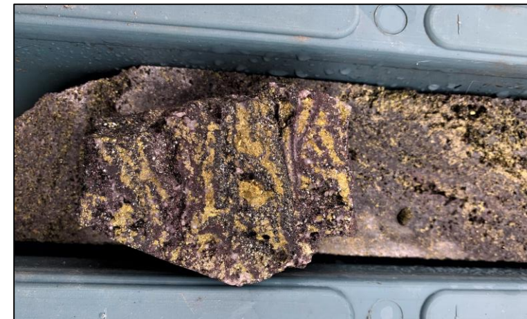
Hematite - specular hematite – magnetite – quartz – chalcopyrite at 423.5m (cut surface).
