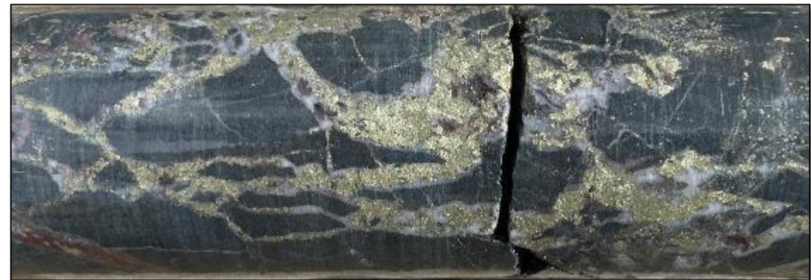
Vein / stockwork-style chalcopyrite+quartz-filled fractures in chlorite+quartz-altered microdiorite. 390.6m.
