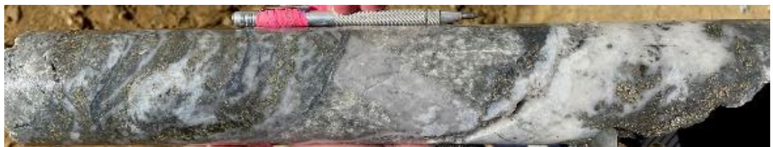
Quartz+pyrite±molybdenite veins overprinting earlier quartz vein in sericite+silica+clay altered Dacite porphyry at 624-624.4m.
