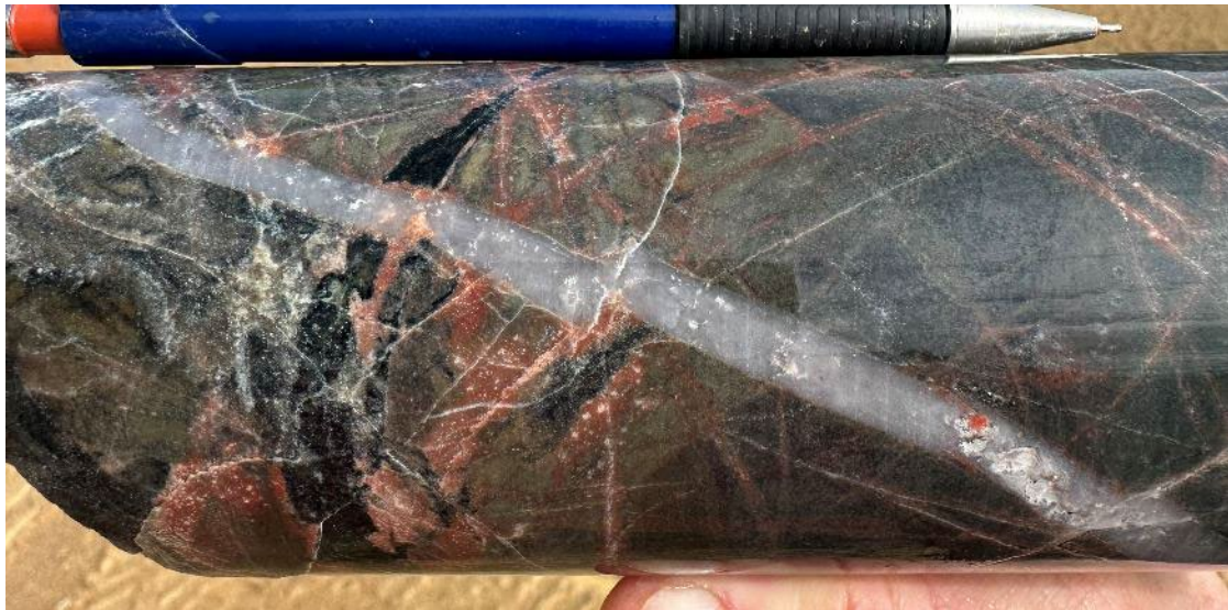
Chlorite+albite+hematite patches cut by quartz vein without selvedge. 779.6m.
