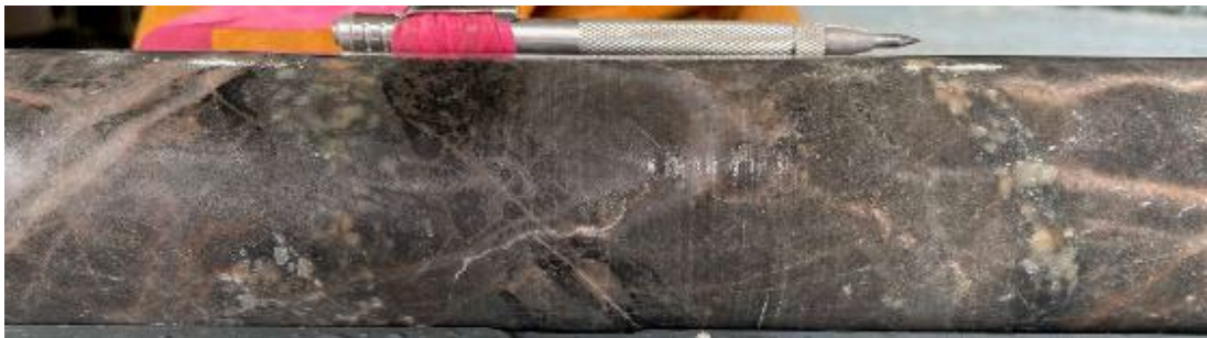
Narrow Dacite Porphyry dykes in sandstone at 661.8m.
