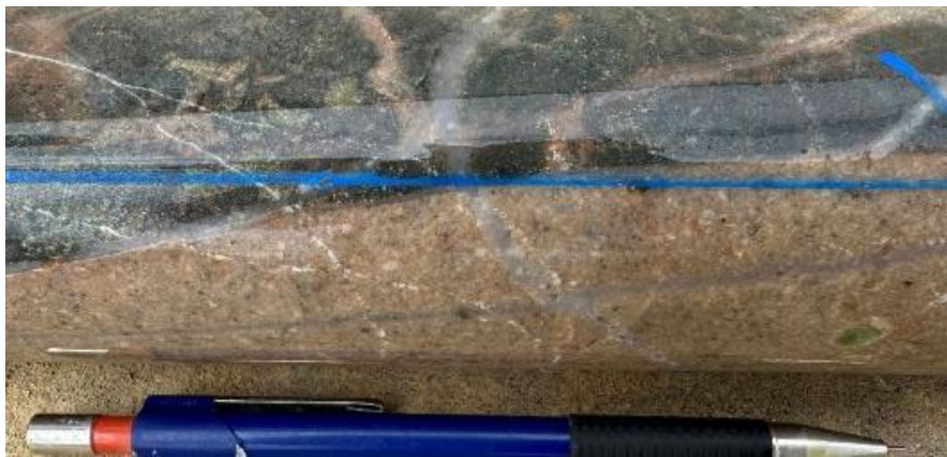
Uphole contact of tonalite / microgranite dyke, cut by younger quartz veins. 450.35m.
