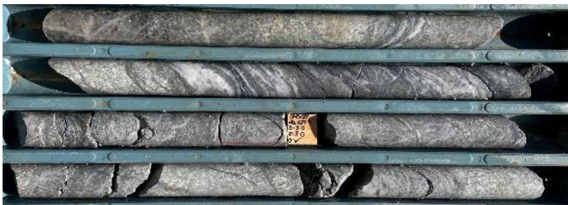
Quartz+pyrite+(trace) molybdenite veins in sericite+silica+clay altered Dacite porphyry from 628-631.1m.
