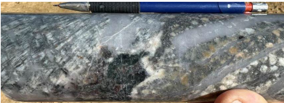
Dacite porphyry. Sub-millimetre sheeted quartz veins (left), a chlorite+muscovite+carbonate+anhydrite patch (centre; screen of host sedimentary rock) and thicker sheeted quartz veins (right). 698.5-698.8m.
