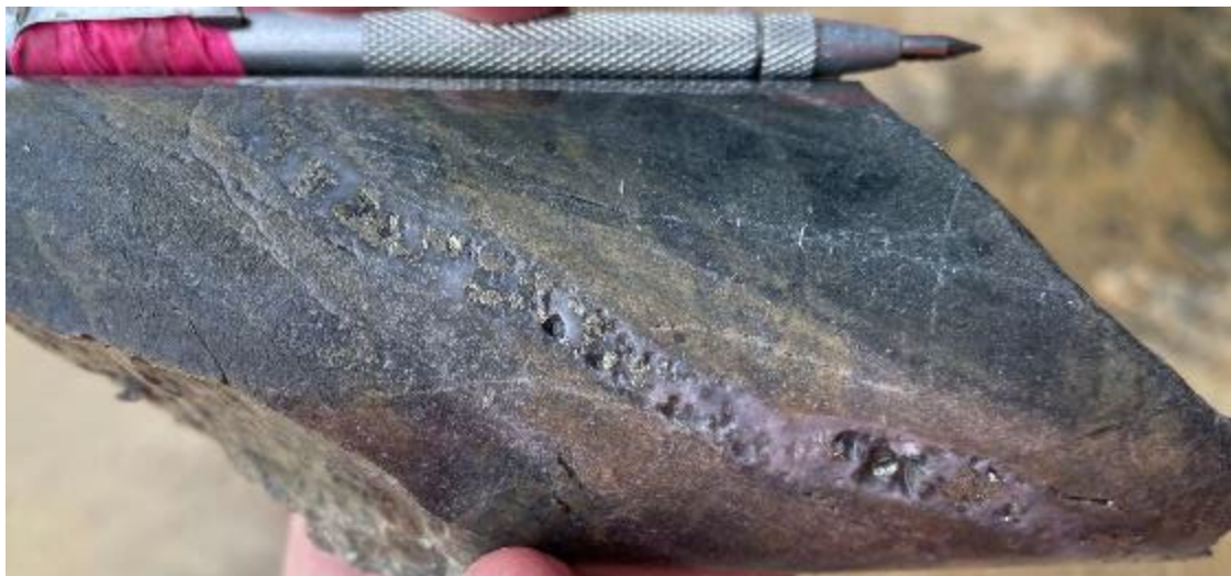
Quartz+pyrite+chalcopryite vein with sericite selvage in sandstone at 299.1m.
