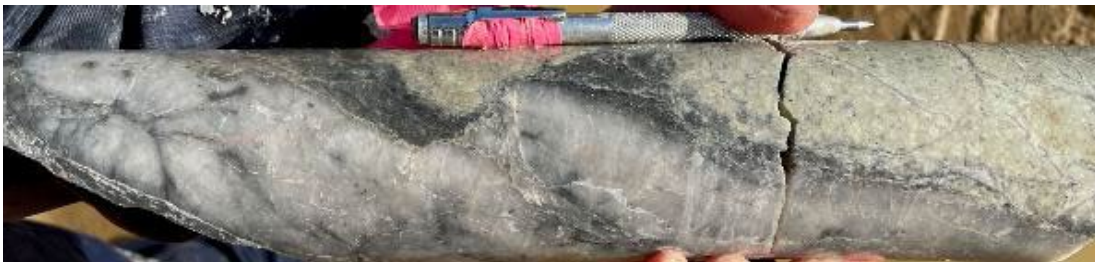
Sheared quartz+pyrite vein at 667.5m.
