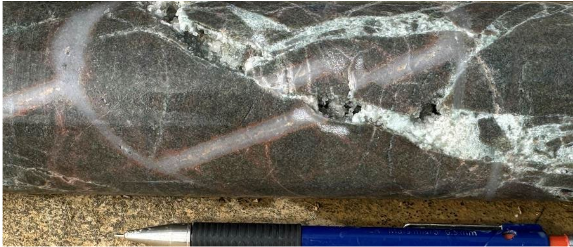
Quartz veins cut by carbonate crackle breccia and fracture-fill. 777.0m.
