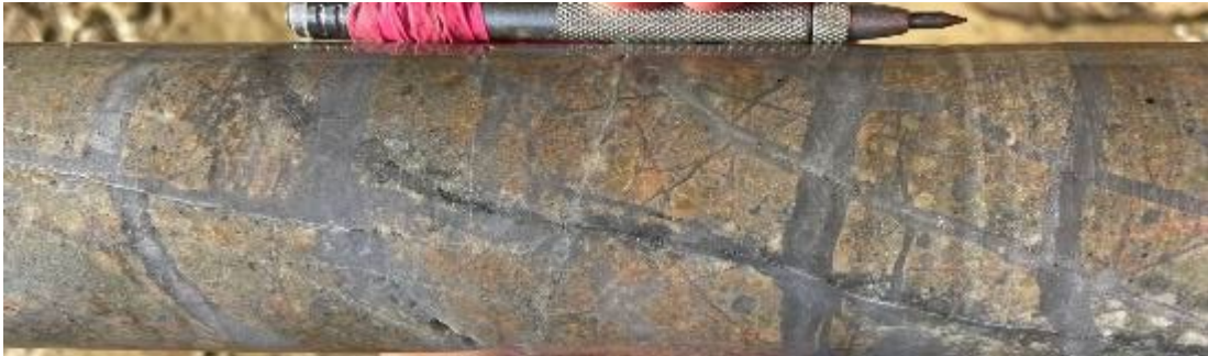
Quartz veins+pyrite centre seams overprinting earlier quartz stockwork veins in strongly sericite+silica+clay altered Dacite porphyry at 579.0m.
