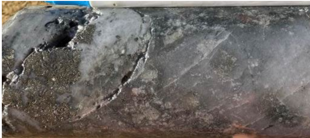
Quartz vein with large pyrite aggregate. 404.4m.
