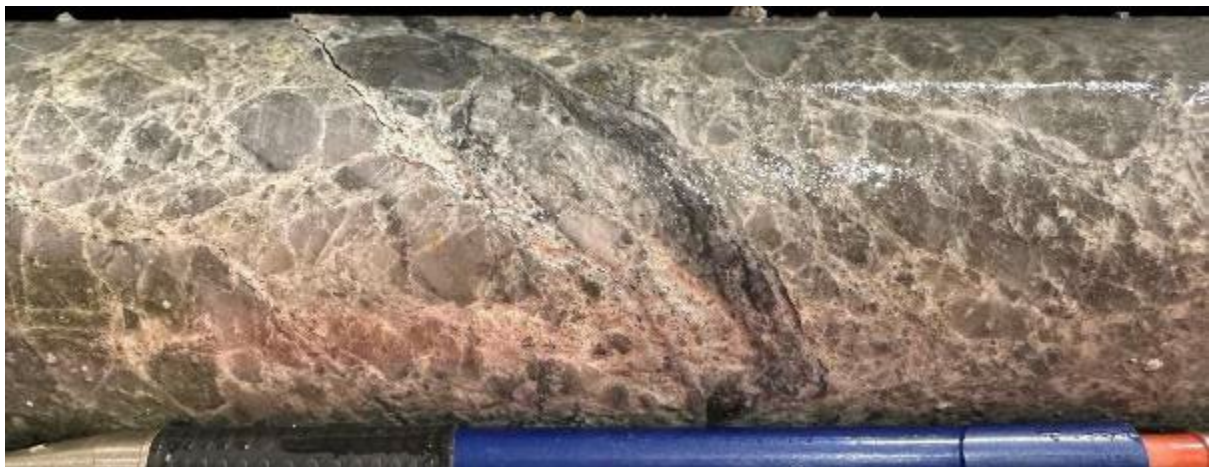
Dacite porphyry. Strong pervasive sericite, cut by brecciated quartz veins (older) and quartz+pyrite veins (younger). 458.1m.
