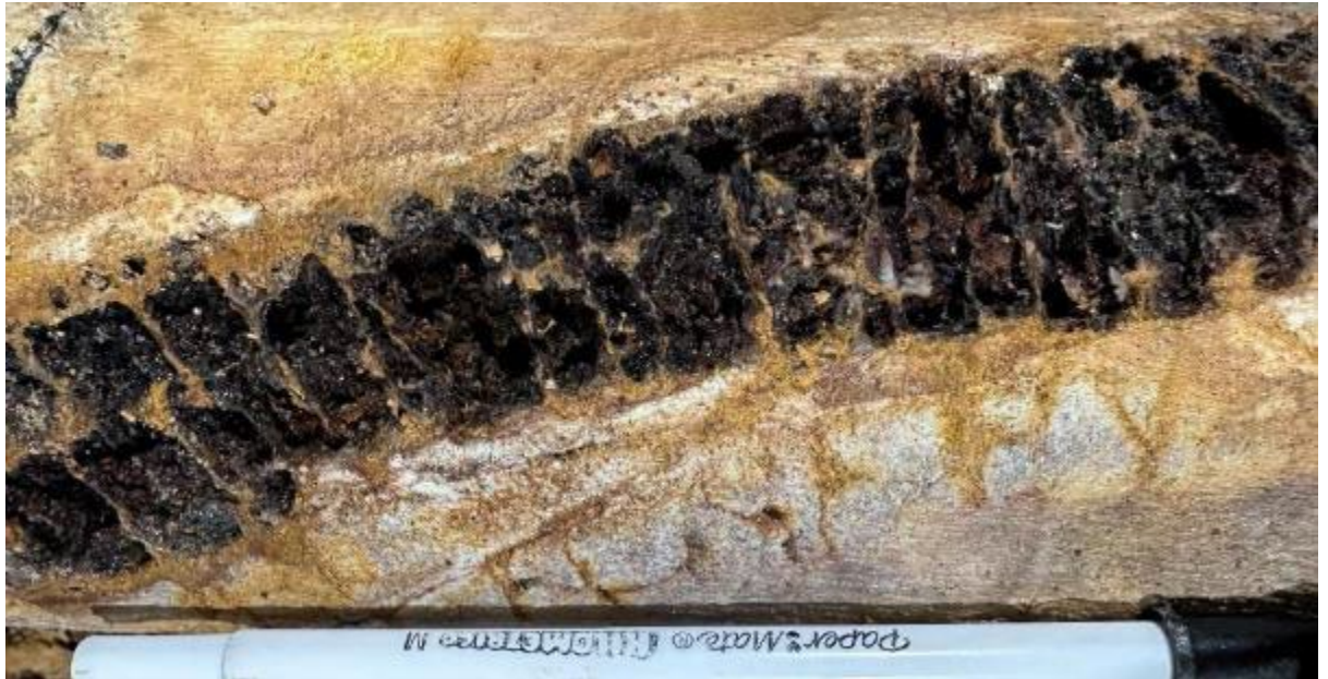
Large hematite+quartz vein in kaolinite-altered sandstone. Probably was a D vein. 30.9m.
