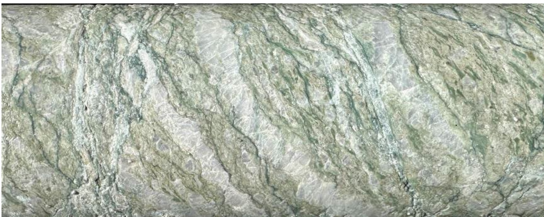
Low Angle Structure. Strongly sheared and sericite+clay-altered dacite. 719.2m.
