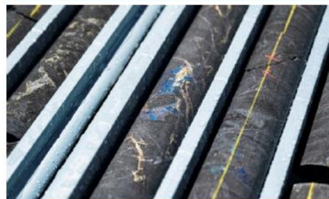
BOD080 - 2m @ 1.01g/t Au and 1.92% Cu bornite-chalcopyrite cemented breccia within 361m @ 0.27g/t Au and 0.15% Cu from 719.7m
