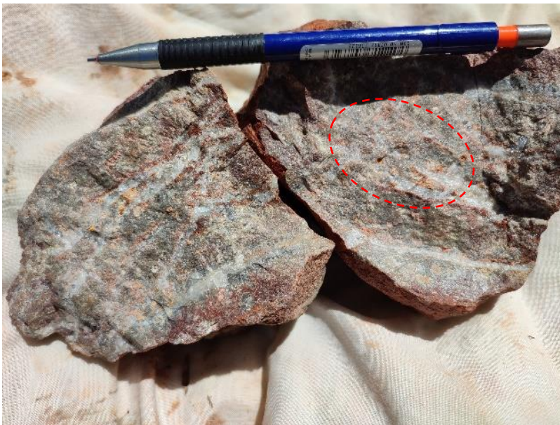
Figure 2: Offset and crosscutting quartz veins indicate development through multiple pulses and support field observations for a large hydrothermal-magmatic porphyry style event at Merino Prospect.
