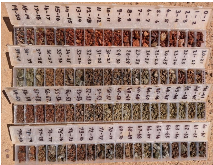
Figure 1 - Chip trays from hole HRC23-008 illustrating areas of propylitic alteration (green minerals) within quartzite from 18m to 79m.
