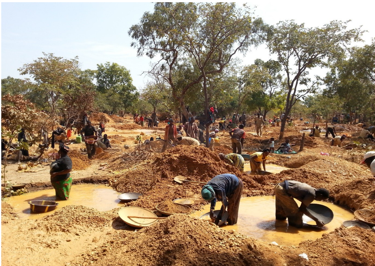
Figure 2: Nangalasso Project – Extensive artisanal workings within the Sotian Concession. Artisanal mining exploiting near surface mineralisation in both transported material and residual bedrock.
