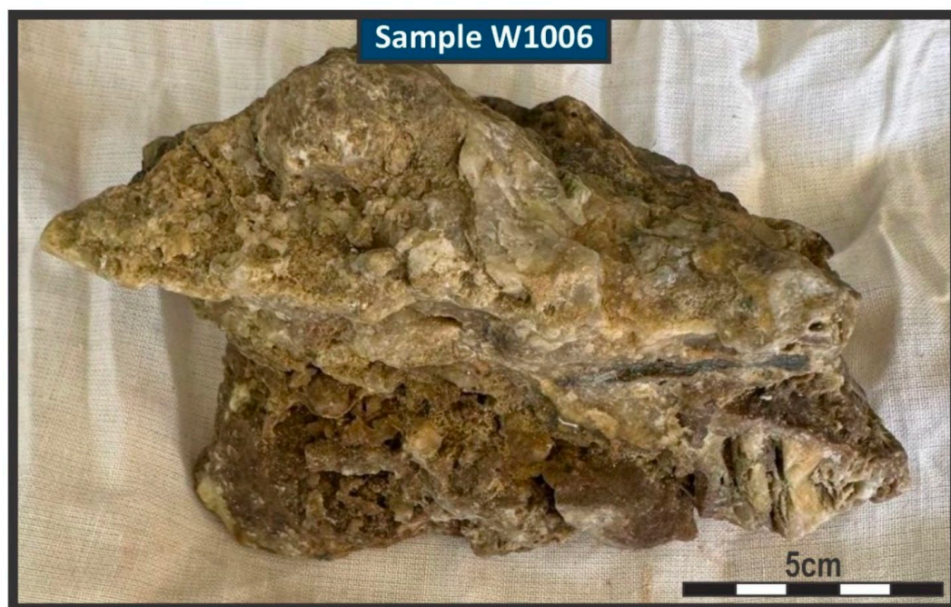
Figure 3: Wenasia prospect float sample – epithermal quartz, sample W1006 – 2.4g/t Au & 82g/t Ag . Location 296739mE / 8891746mN (WGS 84 zone 56).
