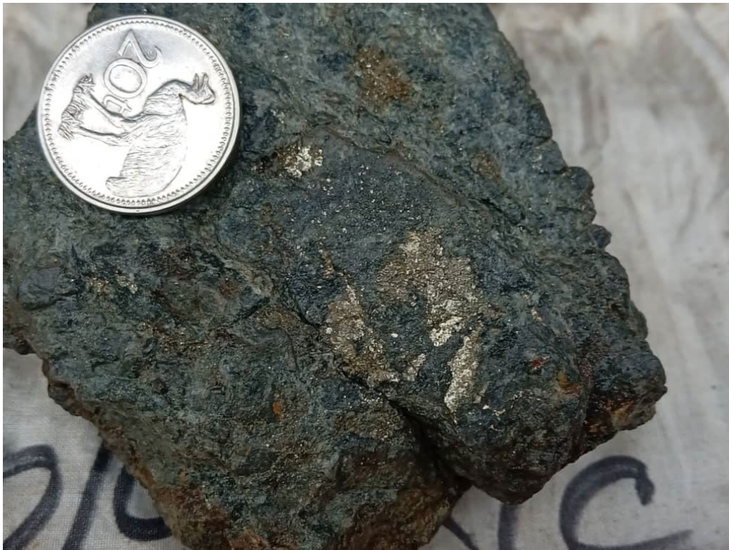
Figure 1: Outcrop Sample 702110 – Visible sulphides in breccia of andesitic volcanic sediment from North access track to Agadul. Visual estimate of sulphides 3% pyrite and 0.5% of fine chalcopyrite.
