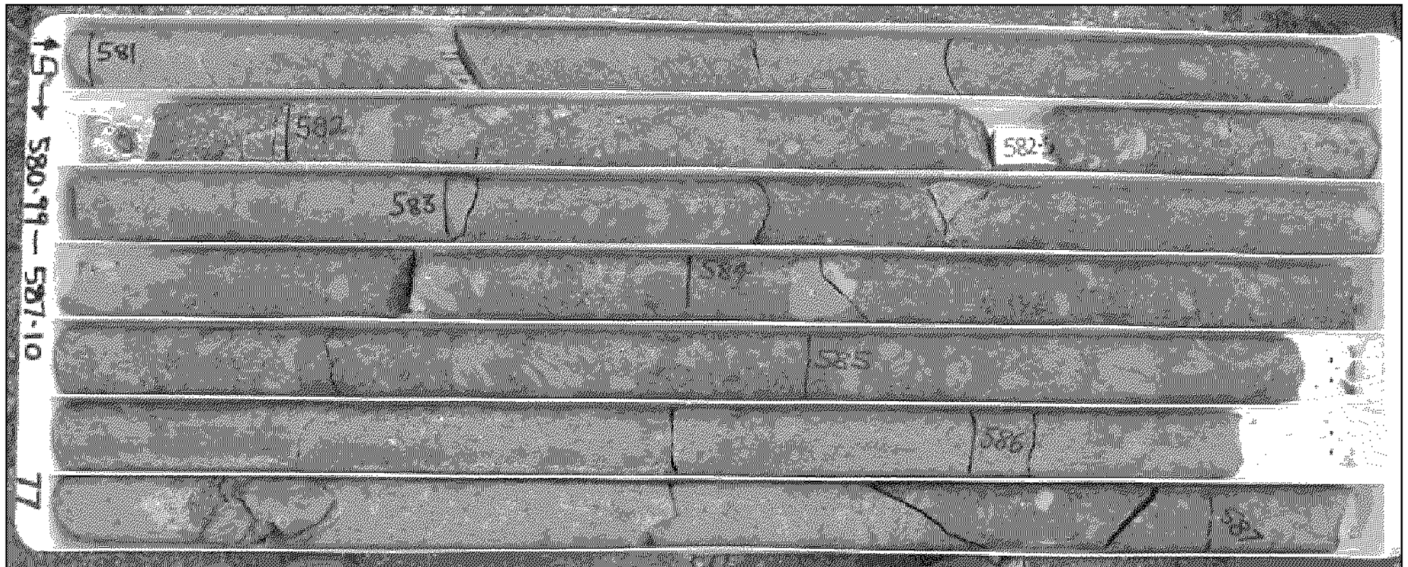
Figure 3: MS 1 drillcore, 580.99m to 587.10m depth. Hematite-rich breccia containing a variety of clast types in hematite-dominated matrix.
