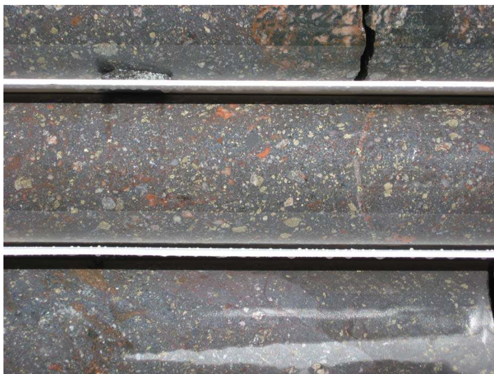
Figure 3: Close-up photo of typical hematite breccia from VUD 7. Hematite is dark grey, sulphides (pyrite and chalcopyrite) are yellow/silverish and the other minerals are carbonate (probably siderite), quartz and feldspar. (NQ Core – approx. 50mm diameter).
