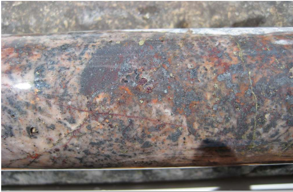
Figure 4: Close up photo of NQ size diamond drill core from 917m depth in VUD 8. Visible is disseminated bornite (purple coloured near centre of photo) chalcopyrite (a different copper iron sulphide mineral, yellow) with associated hematite (grey and reddish) in a very highly silicified breccia host rock. Width of photo is about 15cm.
