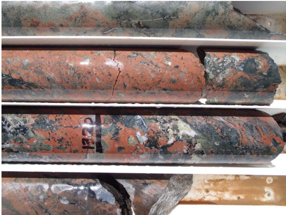
Figure 4: Pervasive “red rock” and variably chlorite-sericite-carbonate altered Wallaroo Group? metasediments hosting chalcopyrite mineralization (yellow) together with pyrite and arsenopyrite? (silvery). Hole LHD002, 1320m NQ2 core.
