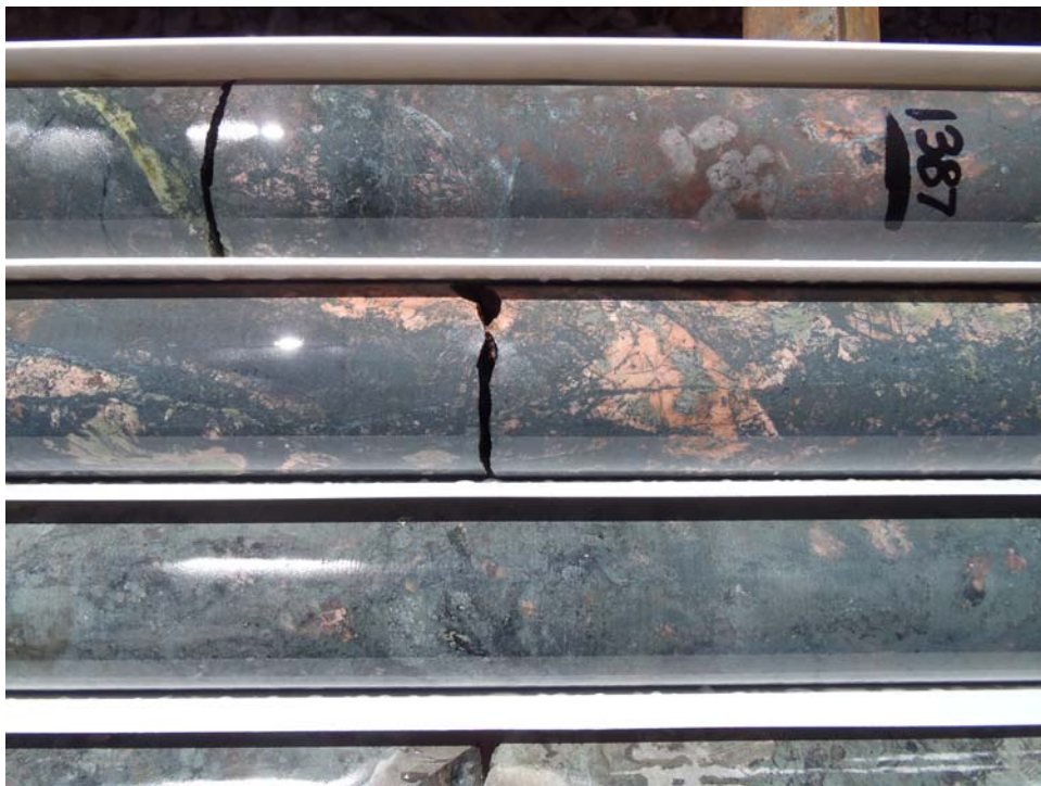
Figure 5: Breccia composed of strongly chlorite-sericite altered Wallaroo Group? metasediments with remnant “red rock” altered clasts. Hole LHD002 1387m NQ2 core.
