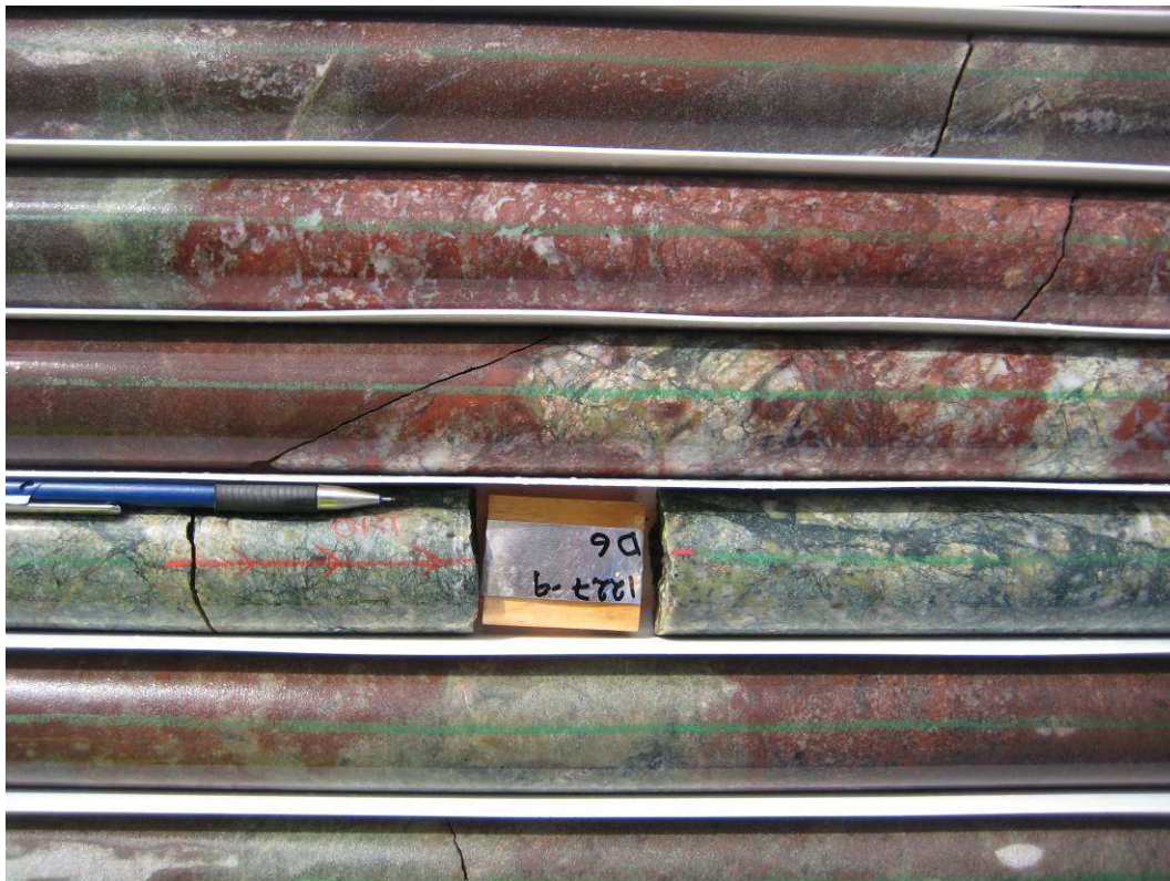
Figure 5a: VUD 13 Approx. 1228m hematite-sericite altered basement rocks (NQ2 core)
