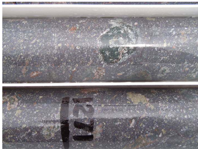
Figure 4b: VUD 12 1271m, pyritic hematite –carbonate breccia (NQ2 core)
