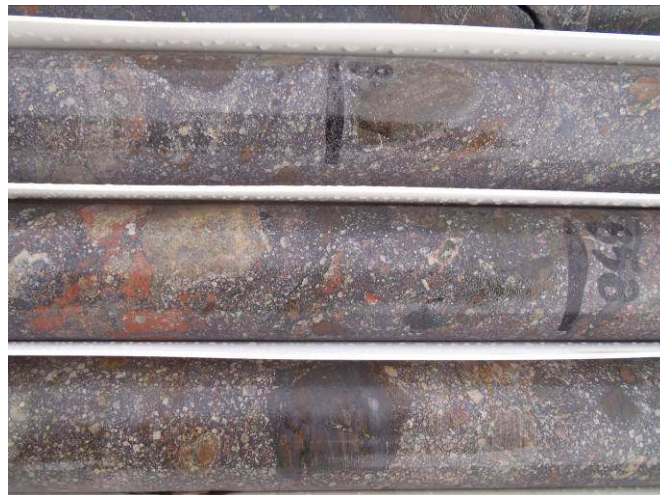
Figure 4a: VUD 12 858m, hematite – carbonate-rock fragment breccia (NQ2 core)
