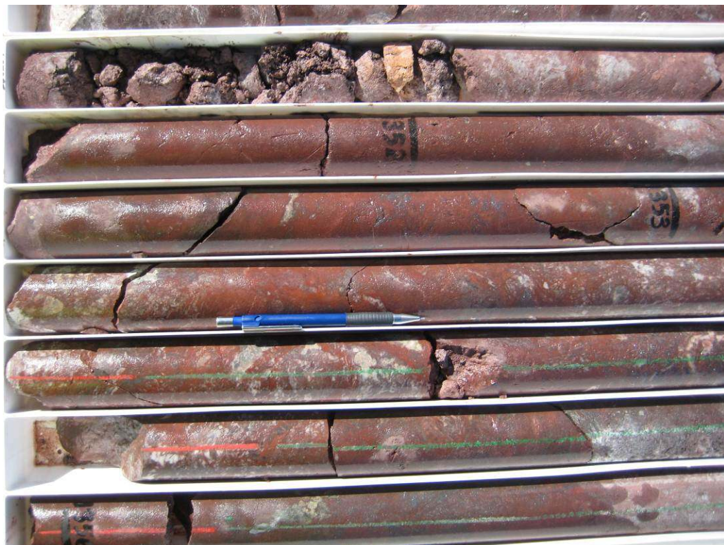
Figure 5b: VUD 13 Approx. 1355m hematite dominated (sericite-carbonate) altered basement rocks (NQ2 core)
