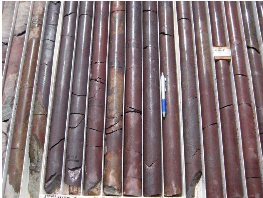
Figure 3b: VUD 11 1029-1040m, massive hematite and hematite-rich breccia (NQ 2 core)
