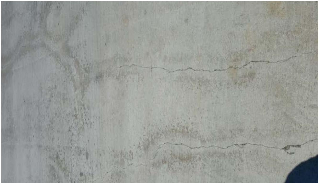
Figure 5. Control Slab Showing Cracking After 6 Months...the EdenCrete™ Slab Showed No Cracking After 6 Months
