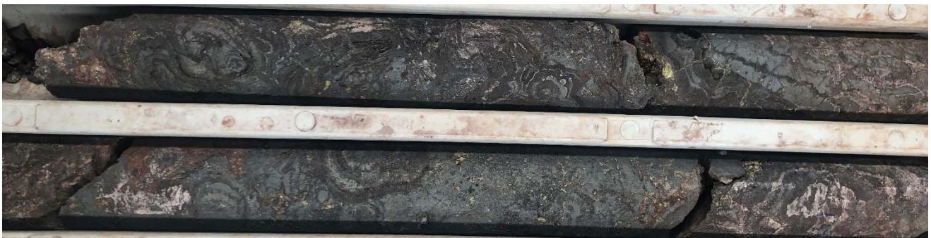
Figure 3: VUD0018, colloform massive hematite breccia at ~1387m, NQ core.
