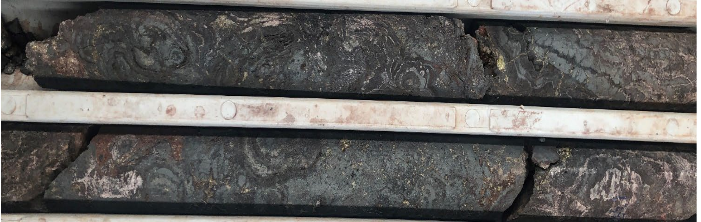
VUD0018 - 1387m. Mineralised coliform massive hematite breccia. NQ2 core.
