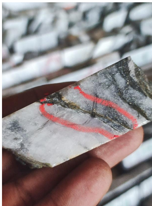
Photo Three & Four | Visible Gold in Anuiri Diamond Core (24ANDDM0004 | 119-120m)
