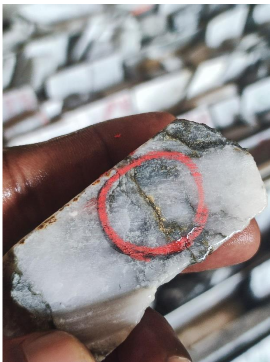
Photo Three & Four | Visible Gold in Anuiri Diamond Core (24ANDDM0004 | 119-120m)
