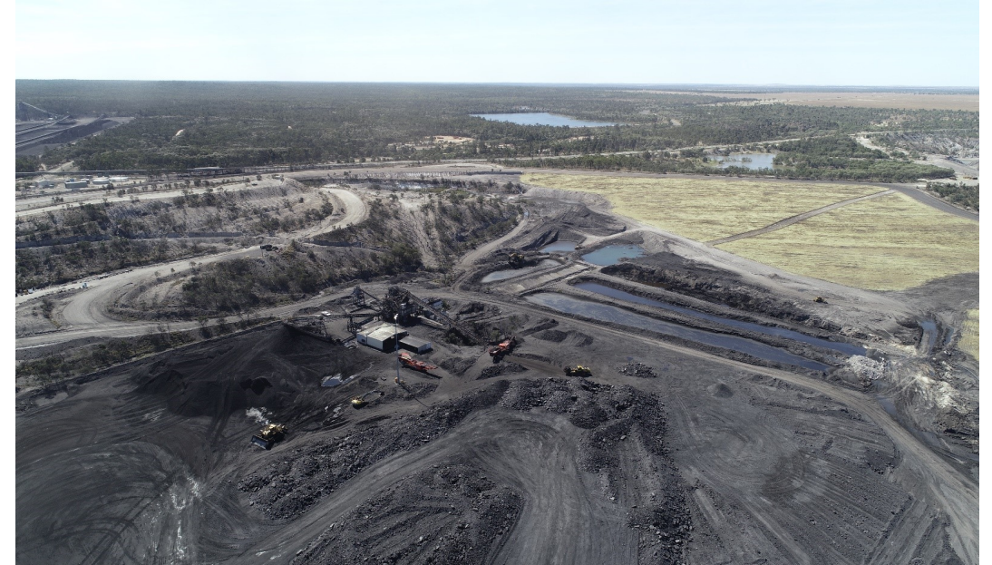
Advancing Face Rehabilitation – South Pit
