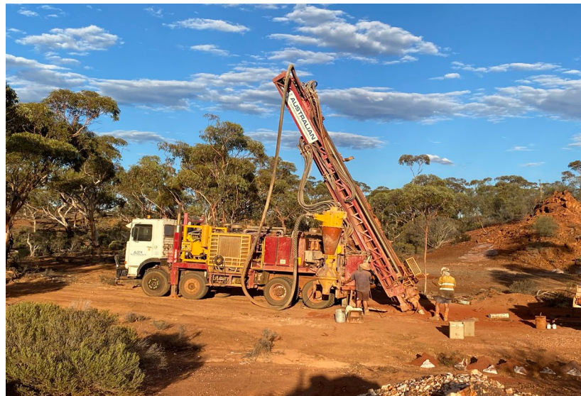
Image 1: RC drilling at El Donna including drill rig and sample piles.
