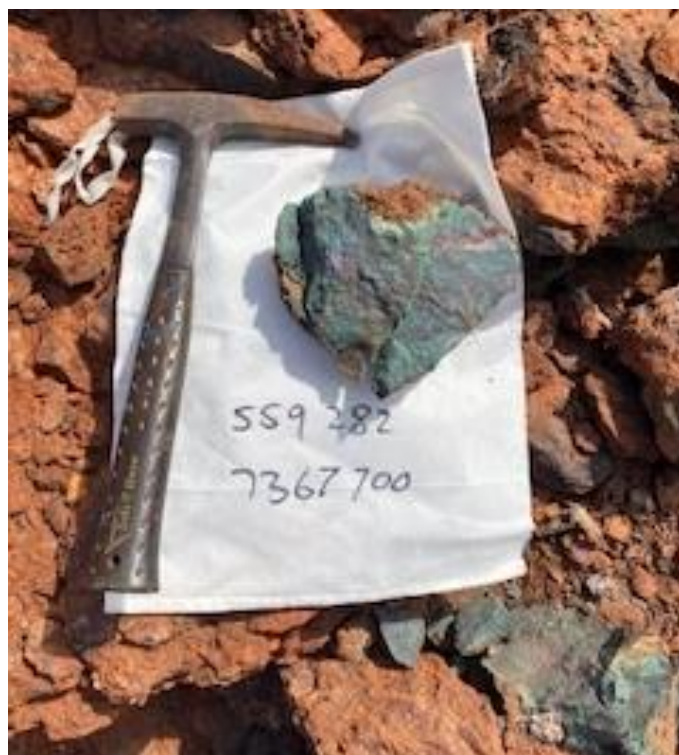
Photo 2: MB274 Copper iron gossan (all from MB1). 31.7% Cu & 0.117g/t Au.
