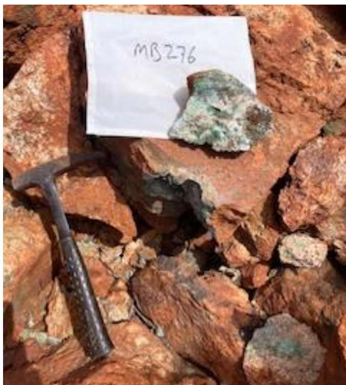
Photo 1: MB276 Hydrothermal quartz, pyrite & malachite (Cu). 1.025g/t Au & 8.08% Cu.
