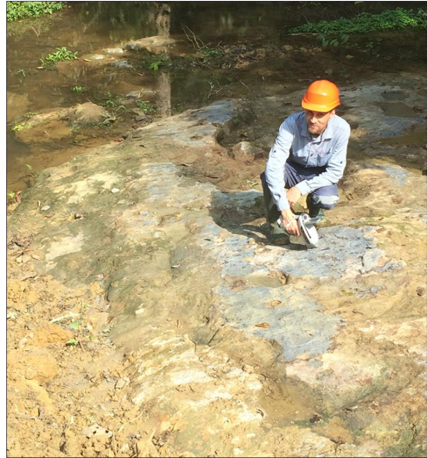
This entire outcrop within the Dikaki embayment contains approximately 20 – 40 % galena and sphalerite (lead and zinc sulphide minerals (respectively))
