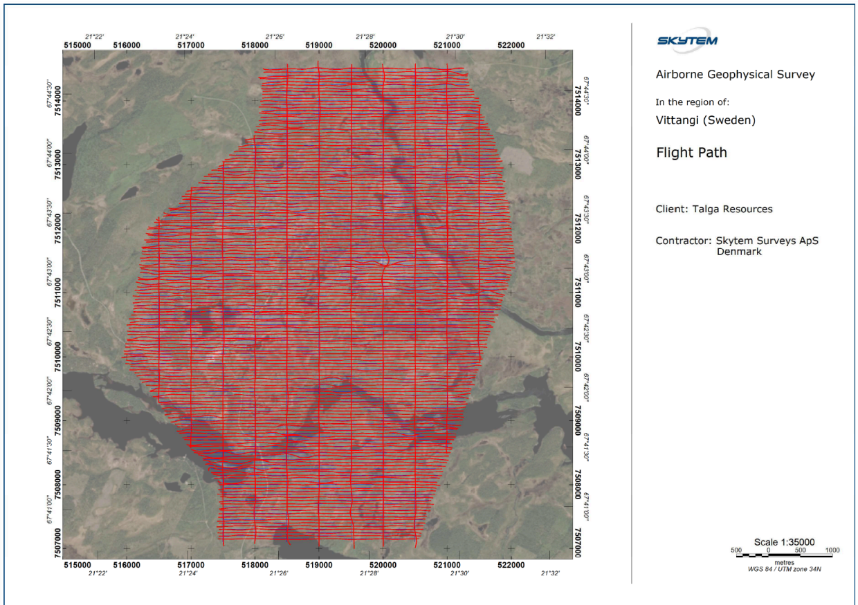
Figure 5 SkyTEM survey flight lines and locations. Vittangi (top) and Aitik East (bottom).
