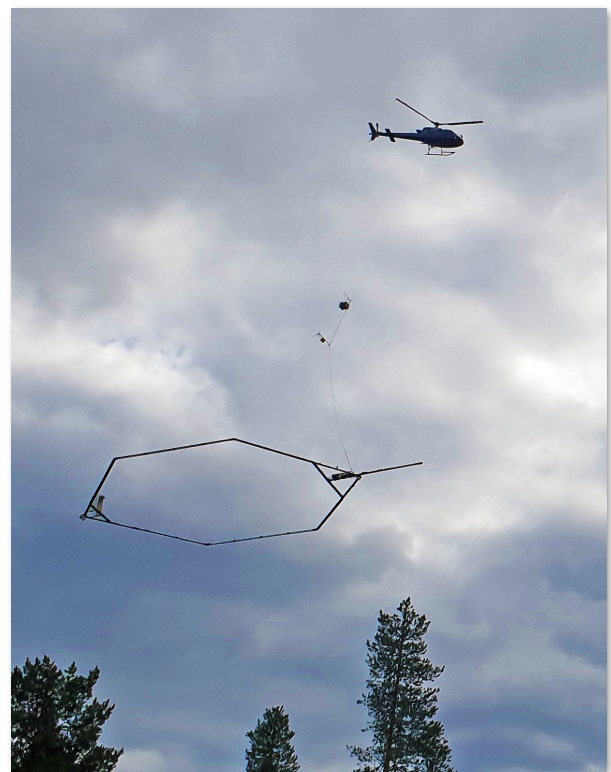
Figure 1 SkyTEM system airborne on Talga project.
