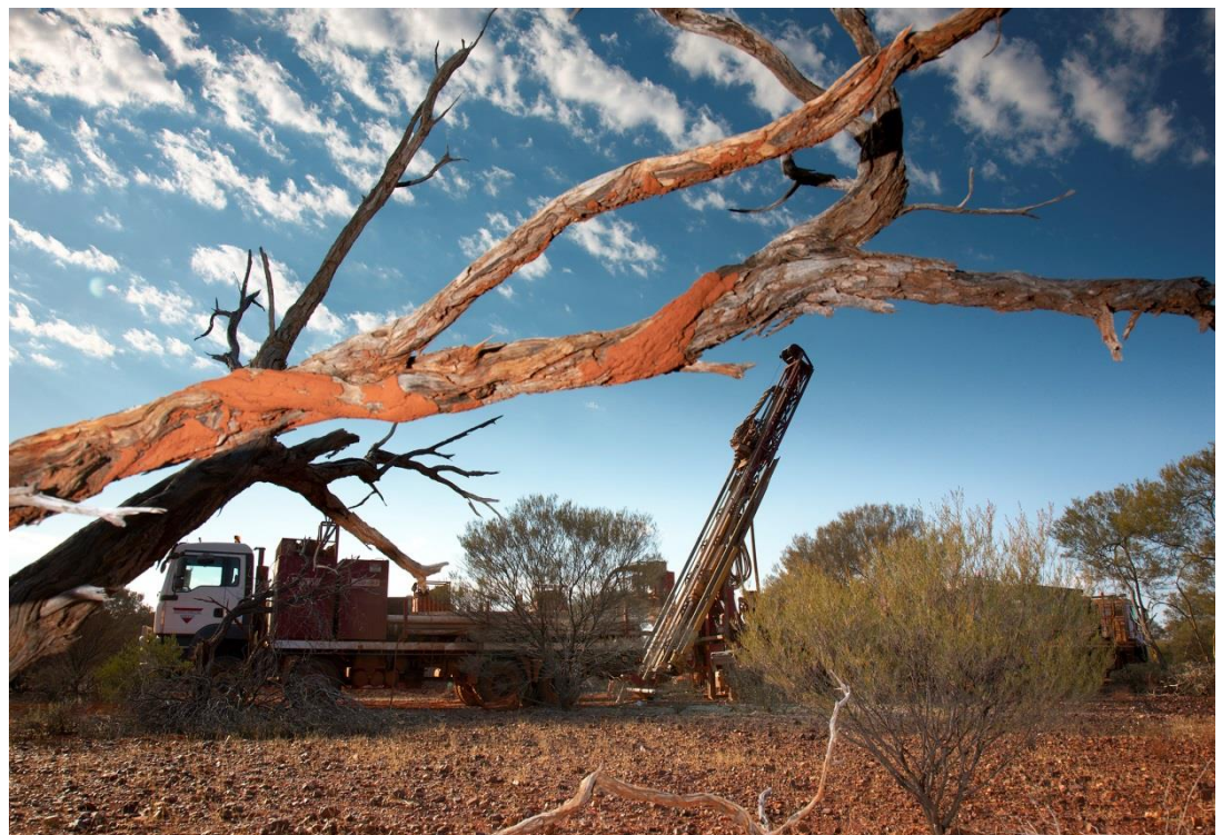
Reverse Circulation Rig at the Springfield Project
