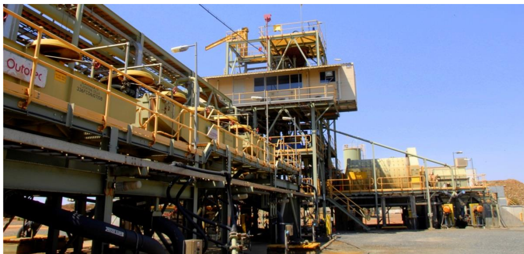
Sinclair Nickel Project: 300ktpa Concentrator – Flotation Cells and Mill Control Room
