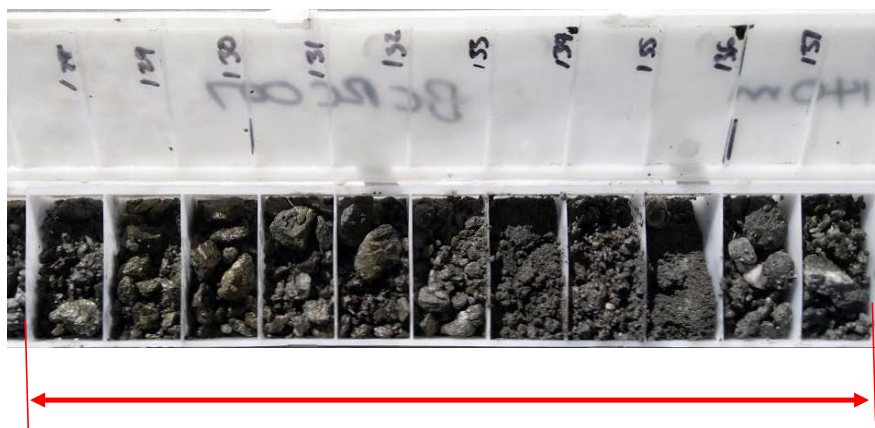
Figure 1: Blind Calf RC drill chips from BCRC007
