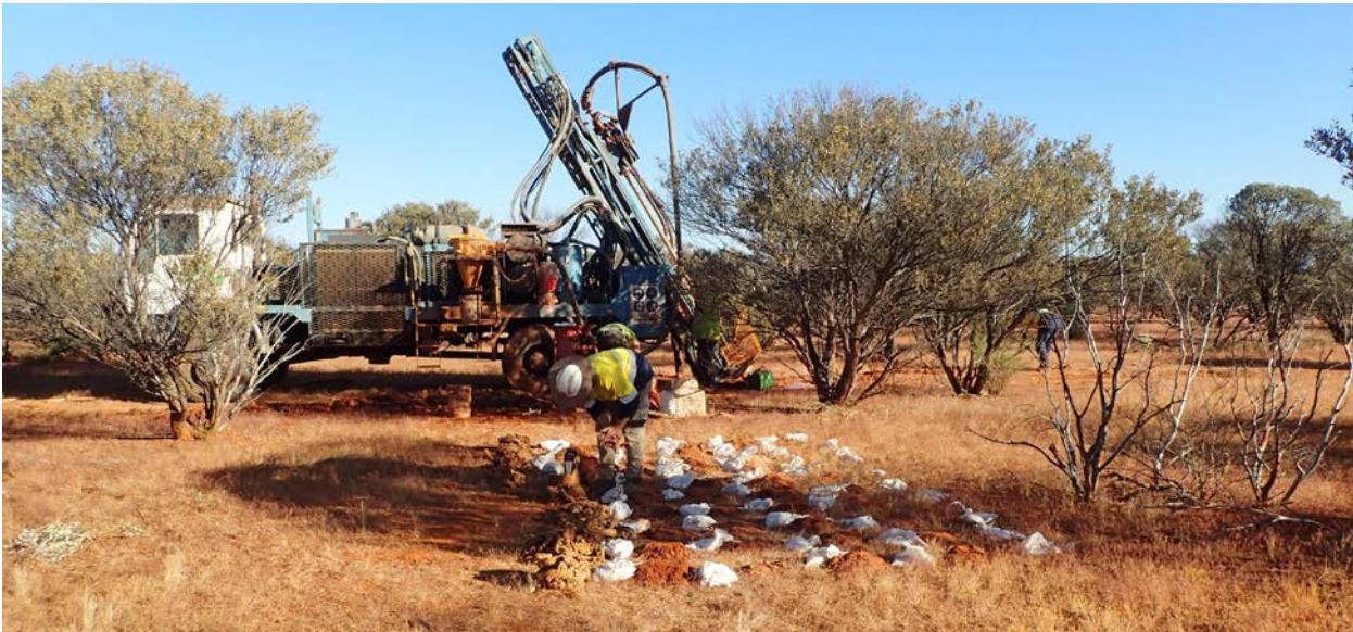
Figure 1: Sinclair Nickel Project – Regional air-core drilling.
