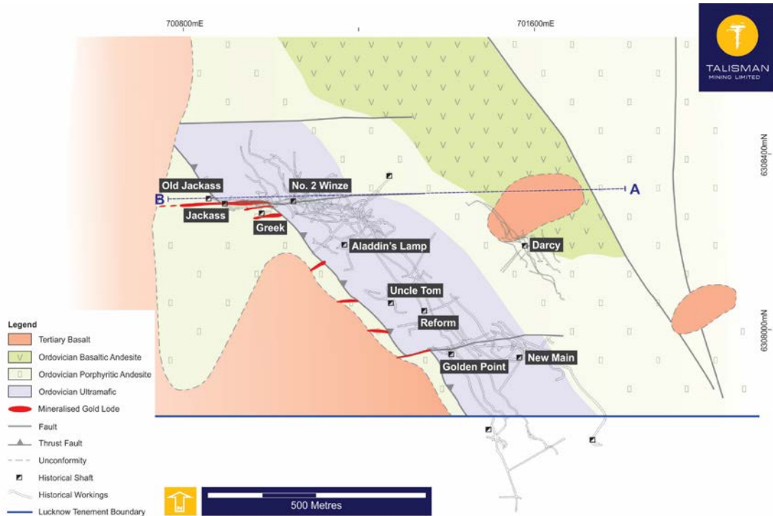
Figure 9: Lucknow Project mine shaft locations and simplified geology.
