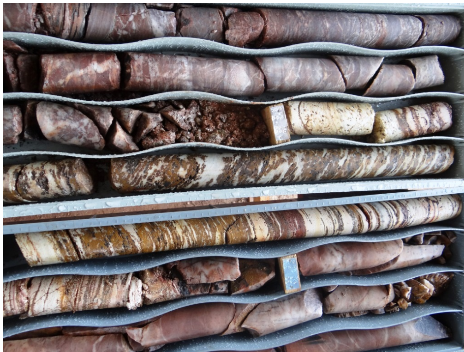
Figure 4: Strong alteration in MID 001-13 from 72.5m to 75.2m
