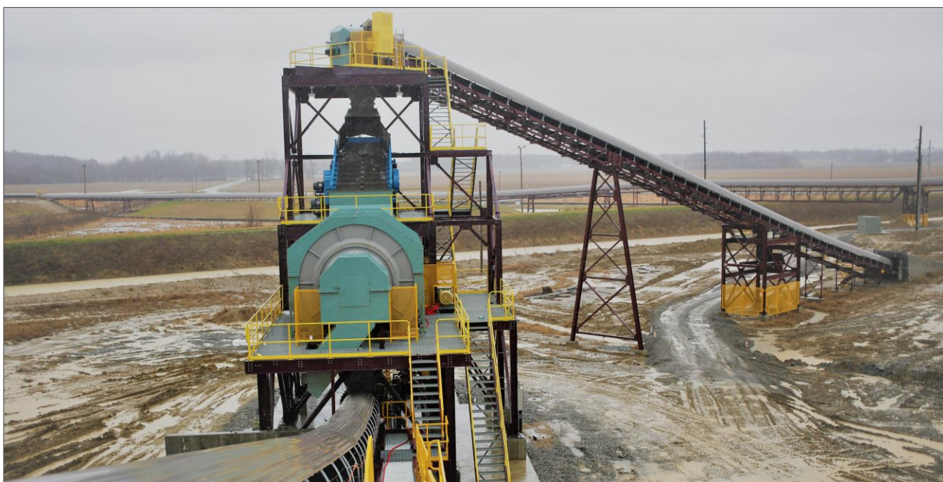
Figure 4: Raw coal reporting to the CHPP ROM screen and rotary breaker
