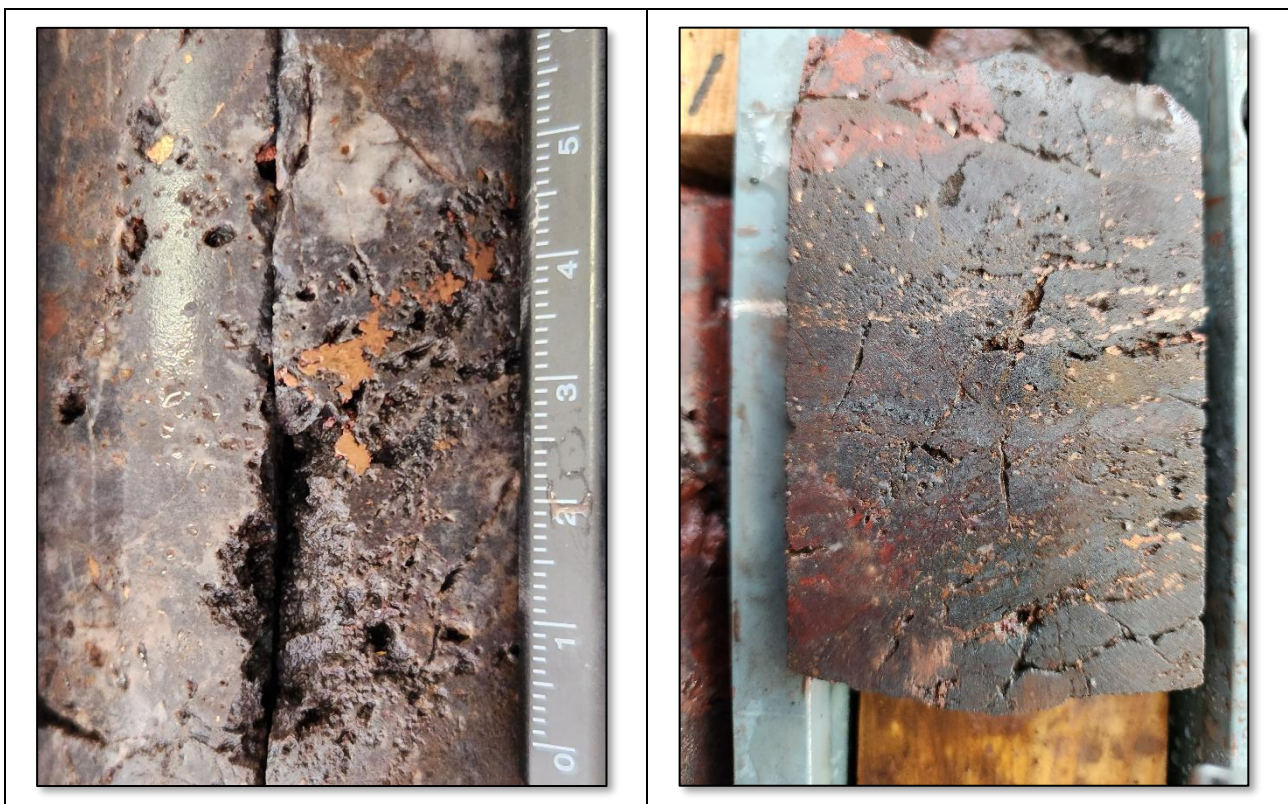
IMAGE 5 a and b: Hematite, quartz, jasper, copper sulphide, copper breccia (BBDD0050 @195m).
