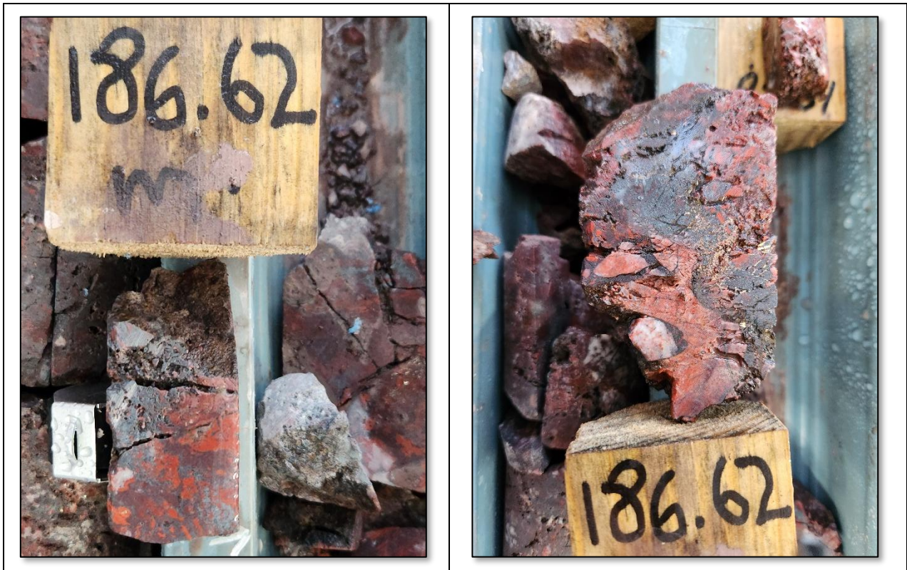
IMAGE 2 a and b: Hematite, quartz, jasper, copper sulphide, copper breccia (BBDD0050 @186m).
