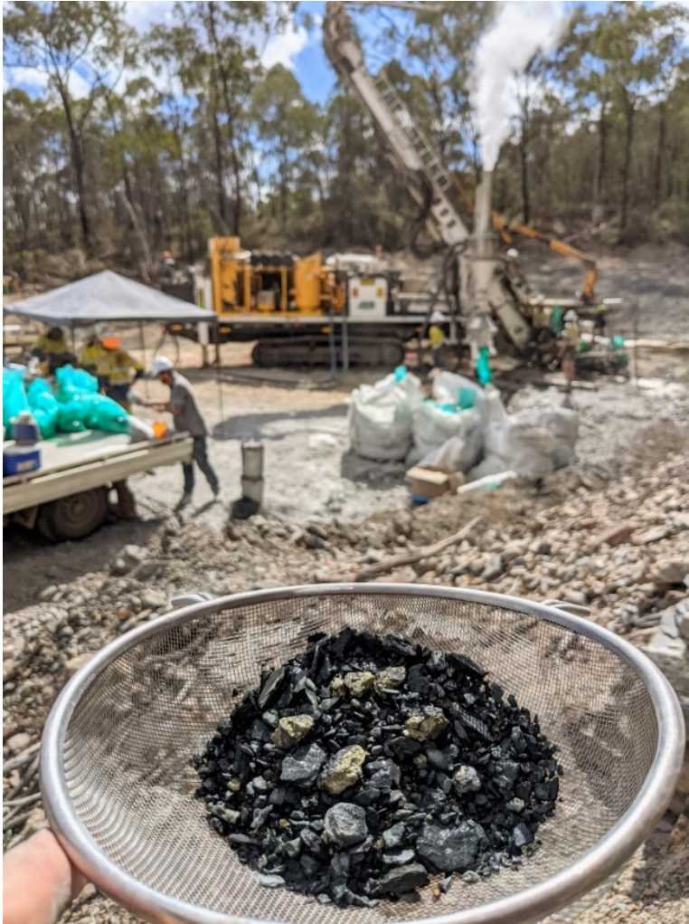
Figure 6. Chalcopyrite logged from drilling at Quorn.
