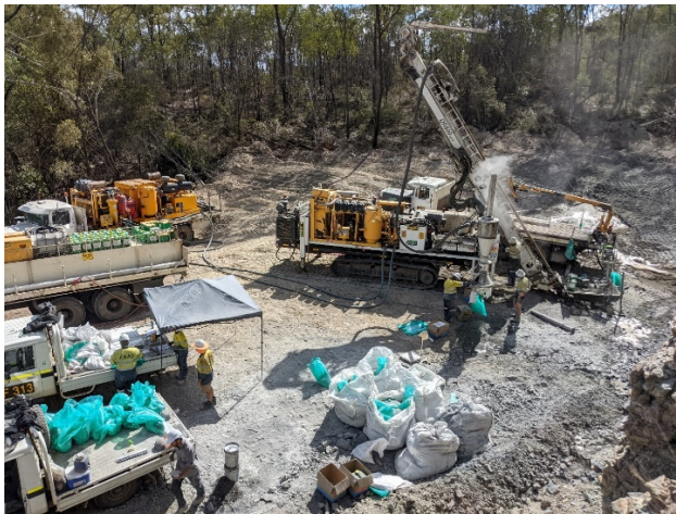
Drilling first exploration hole at the Quorn prospect and logging system for exploration drilling at Quorn analysing sample chips, using pXRF.
