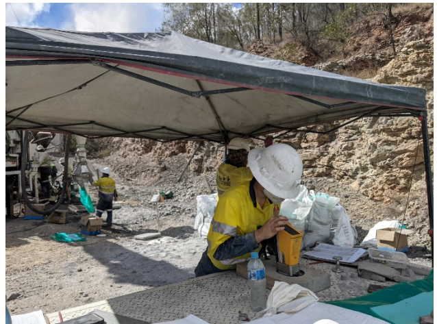
Drilling first exploration hole at the Quorn prospect and logging system for exploration drilling at Quorn analysing sample chips, using pXRF.
