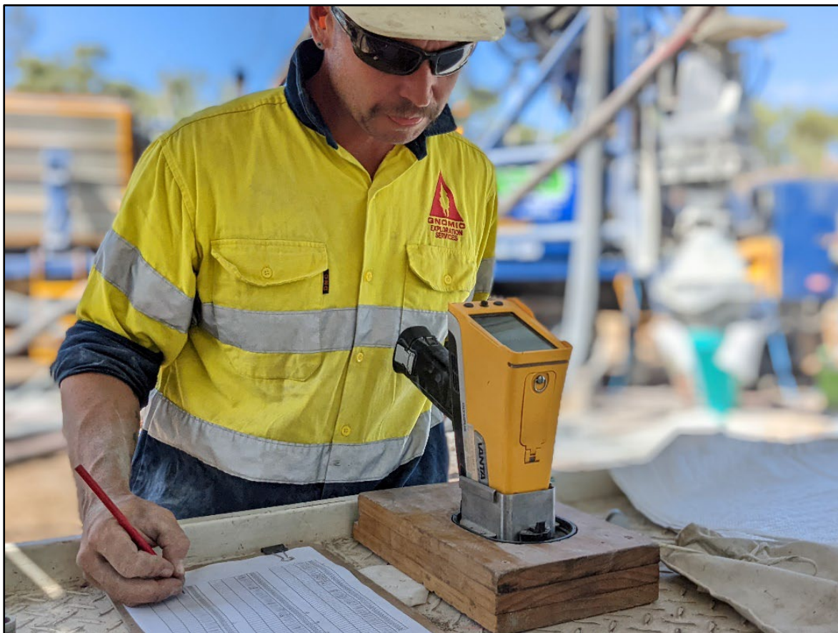
Figure A1: pXRF Vanta m-series analysing a sample at the drill rig to provide rapid indicated mineralisation grades.
