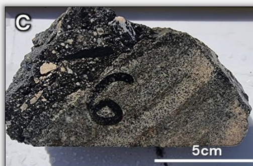
ECDD002: 66.58 to 66.67m Interpreted streaming textures in rockflour breccia
