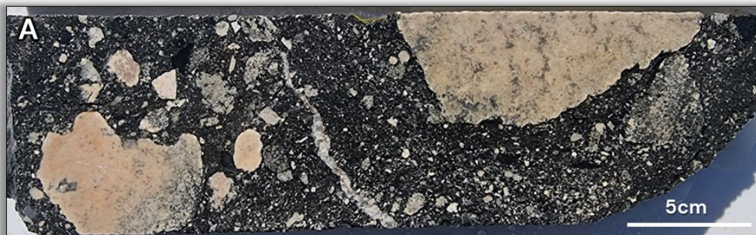
ECDD002: 57.00 to 57.22m Interpreted phreatomagmatic breccia with juvenile clasts of fine grained felsic intrusive in biotite altered breccia matrix
