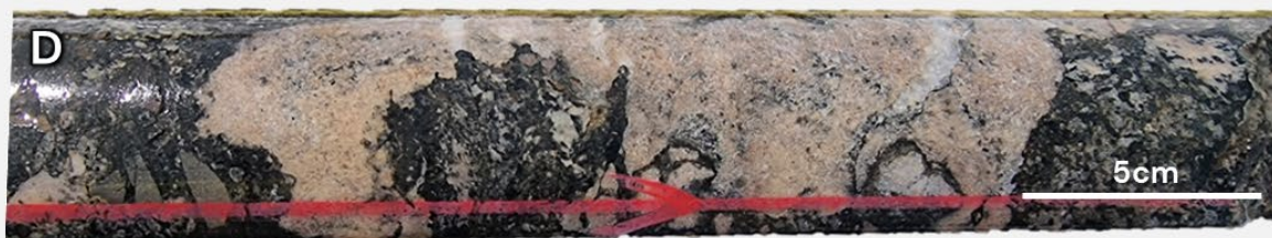
ECDD002: 137.55 to 138.0m Felsic dyklet intruded into originally unconsolidated phreatomagmatic breccia
