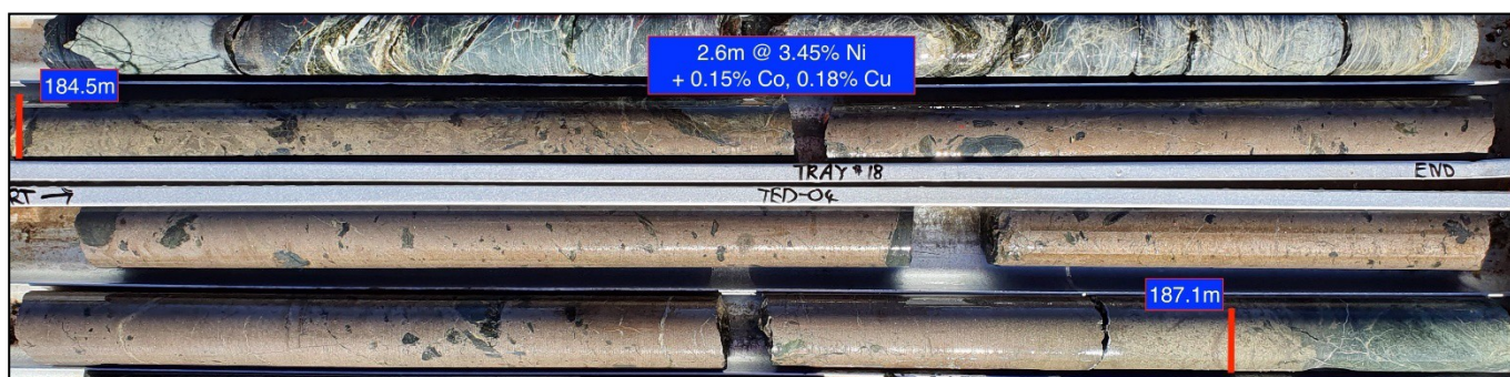
Figure 4: Photo of massive nickel sulphide intersection in diamond hole TED04, the second diamond hole drilled at the Dusty Nickel-Gold Prospect.
