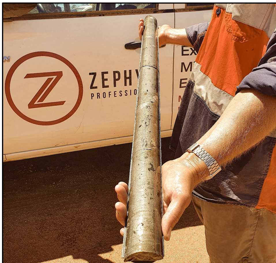
Figure 1: Photo of massive nickel sulphide in drill core of diamond hole TED07 at the Dusty nickel discovery on Toro's 100% owned Yandal Gold Project – this part of the core grades 4.01% nickel (see text for details).
