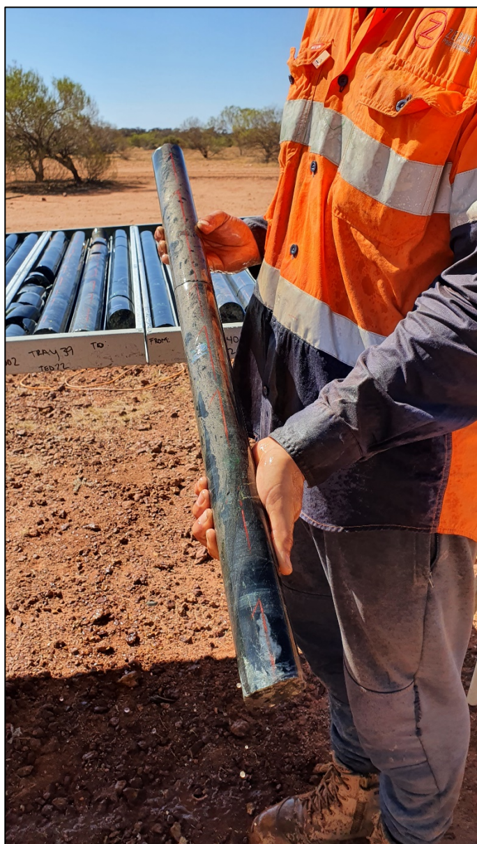
Figure 1: Lens of massive nickel sulphide intersected in diamond drill hole TED22 at Dusty 1. See text for further details.
