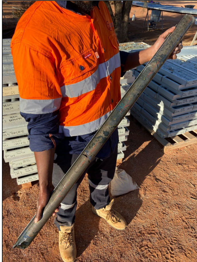
Figure 1: Diamond drill core of massive & semi-massive nickel sulphide intersected in TED38.
