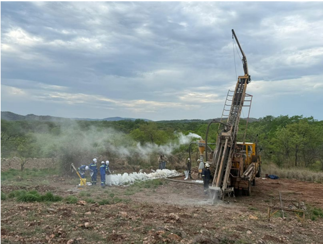
Figure 1: RC drilling underway at Aucu at the Chewbacca prospect, targeting quartz–sulphide–alteration structures within near-surface volcanic and intrusive units. Sample bags align in preparation for geological logging and assay submission.
