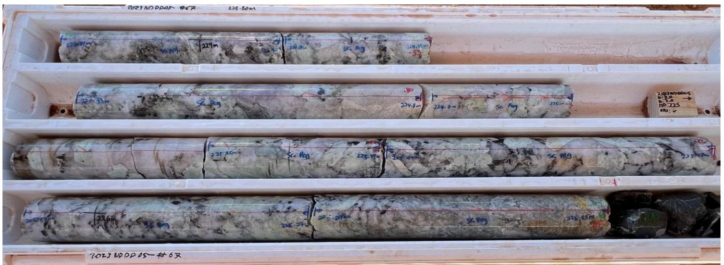
Figure 4 Diamond core 23NDD005 from 223.81m to 226.7m from New Dawn Lithium Project. Note that assays for this hole were received.
