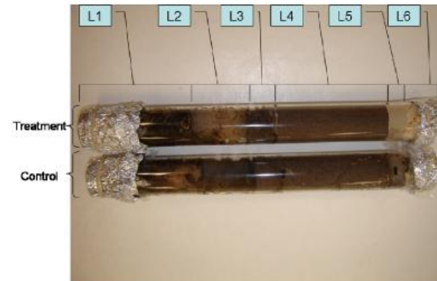
Fig 2. Set-up of vertical assay tubes (22 mm diam. x 190 mm) (modified after Su et al.1995)
