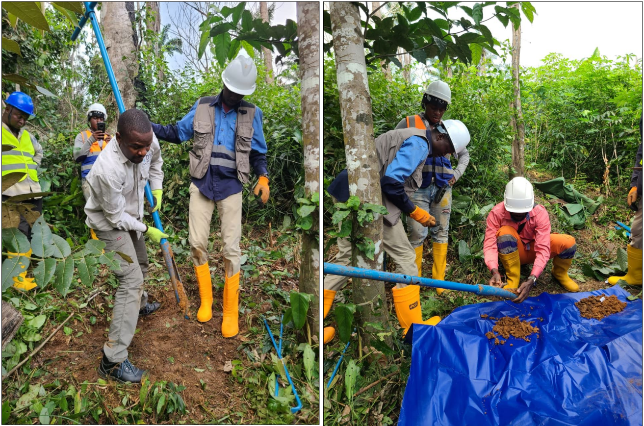
Figure 3: Tusker Minerals hand auger drilling activities showing sample collection process.
