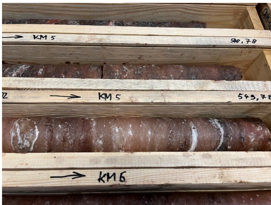
Figure 2: Overview of core recovery, boxing and depth logging. Excellent core recovery and overall condition is being achieved as evident from the photographs.
