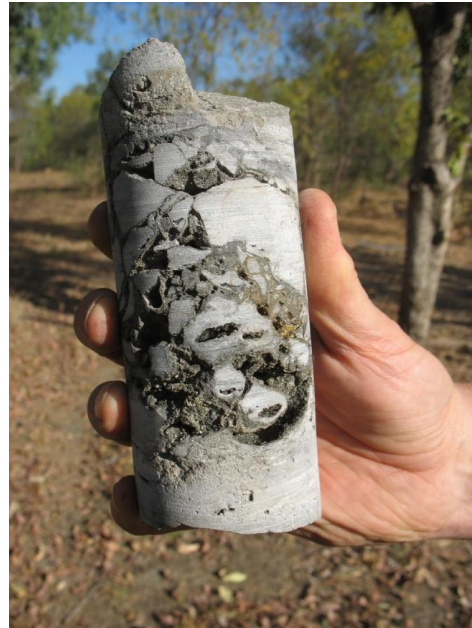
Plate 2: Sphalerite in replacement breccia, BDD002
