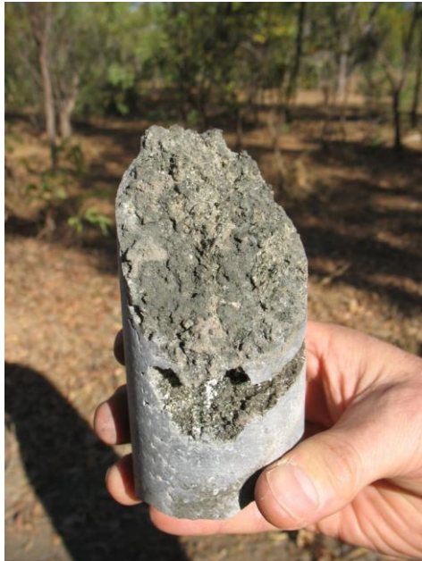
Plate 1: Sphalerite on vug and fracture plane, BDD001
