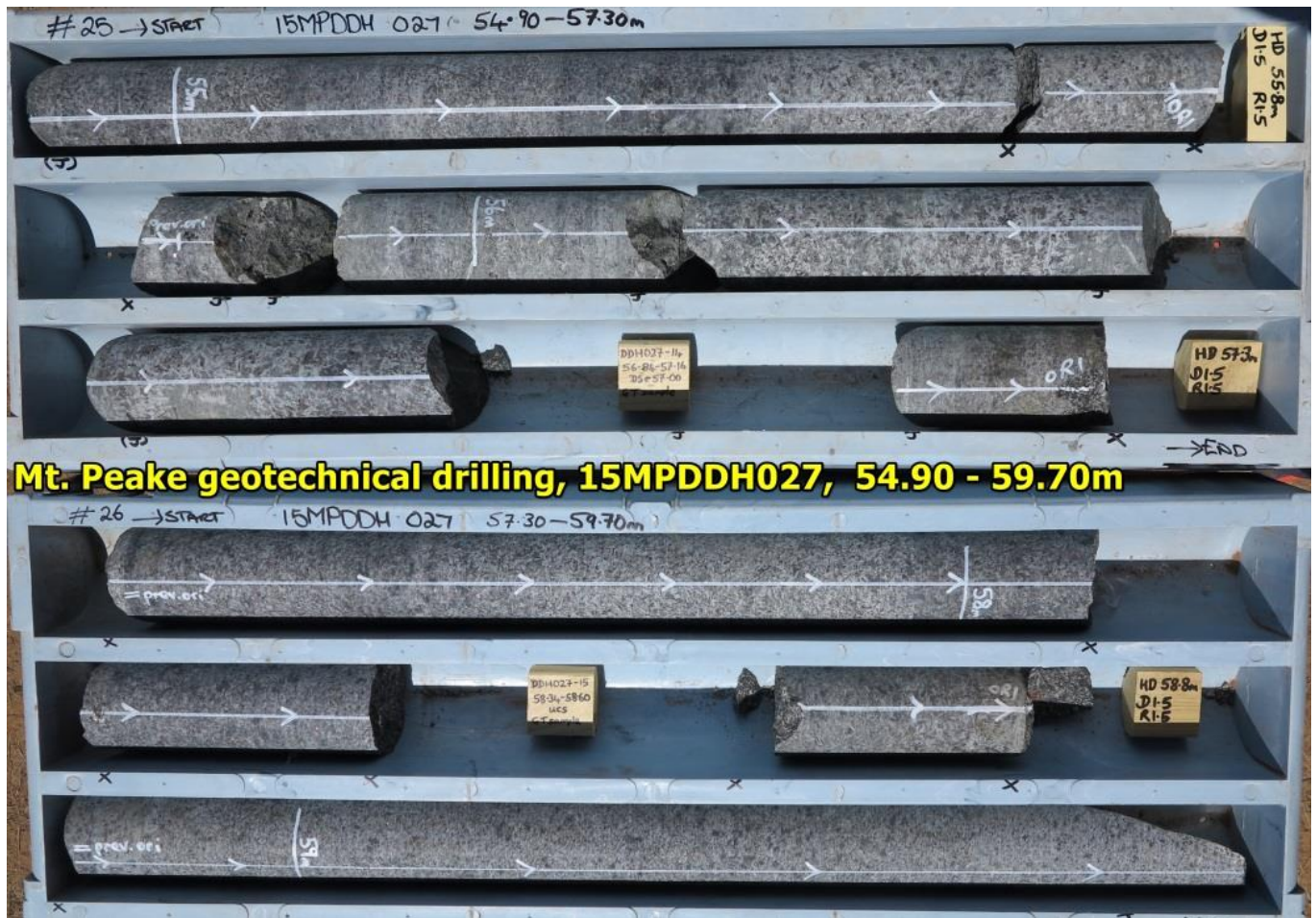
Figure 2. Core tray photograph, showing oriented competent coarse-grained and unaltered hangingwall gabbro from the central eastern part of the resource.
