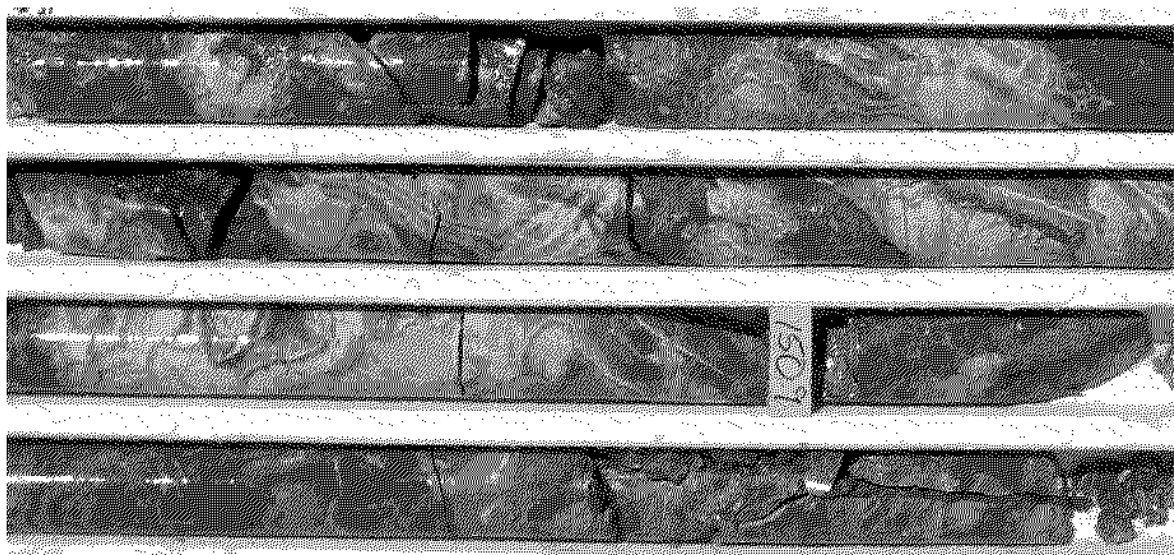
Typical fine-grained Pb-Zn mineralisation from recent drilling at Menninnie South (MD66 @ ~150m HQ core)
